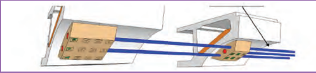
Figure 5: the blister is attached to the existing bridge deck as an anchor or guide for the new post tensioned cables
